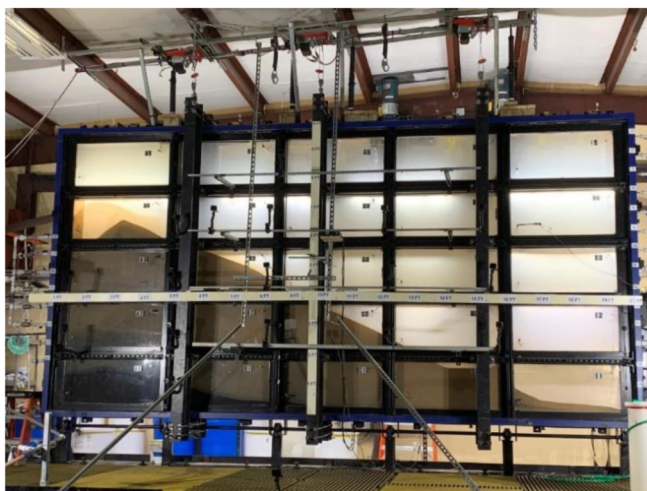
Figure 5—10 ft. × 20 ft. Slot Flow Test: Mid-Test Photo Showing Settled Dune & Proppant/Fluid Moving Left to Right
